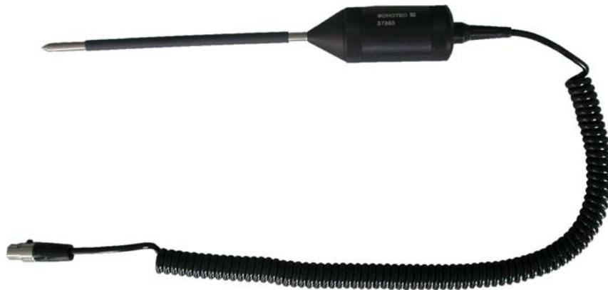
They have to be pressed onto the testing place by hand. Favourable points are those, where within the stream trap flow transitions are arising.
