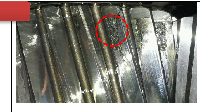
Actual Gear damage as viewed at inspection May 1, 2013
