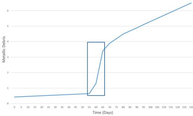
Sensor reading when coarse debris is detected
