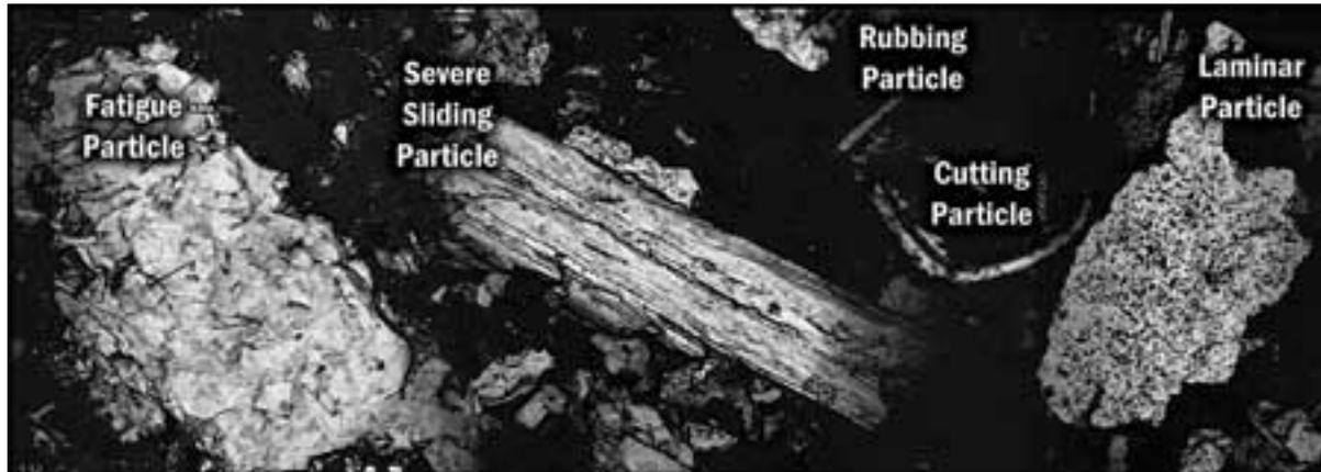
Wear particles generated from component failure.
