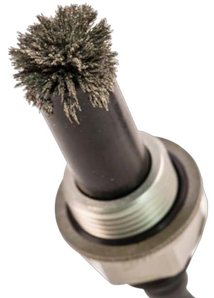
Sensor reading when fine debris is captured
