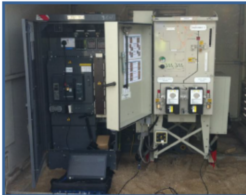
PrecisePD being used to test the RMU
