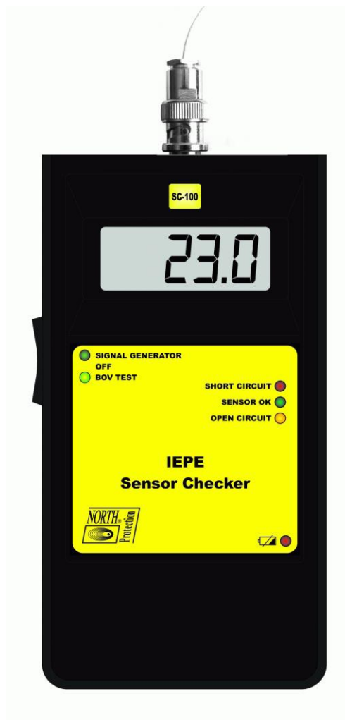
Figure 8: High Bias Voltage Indication
