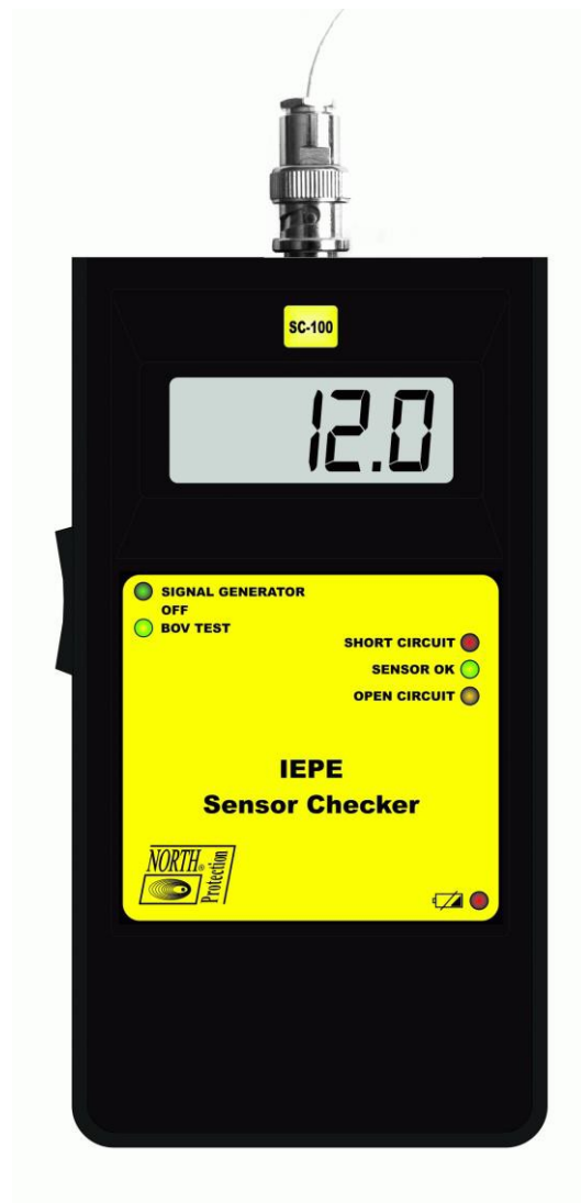
Figure 7: Good Bias Voltage Indication
