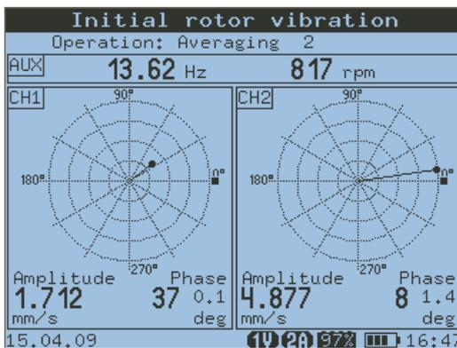
Balancing: Initial rotor vibration
