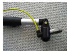
Shows 3 of an infinite number of available sensor angles (auto adjust) simplifying the attachment of sensor/magnetic mounts to any machine
