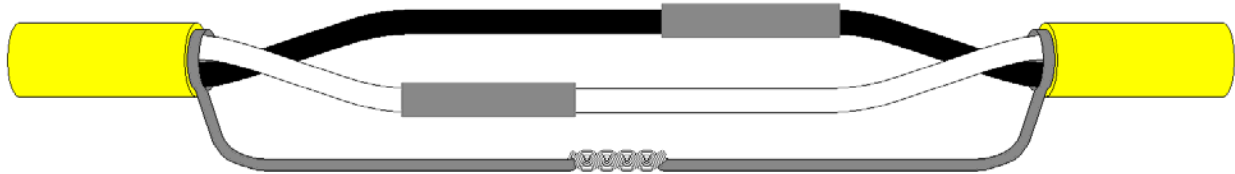
Figure 3 - Apply shrink tubing or tape to each of the twisted conductors to insulate the connection
