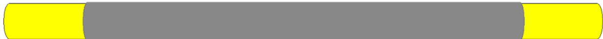
Figure 5 - Apply insulating tape to the outer jacket along the entire length of the splice. Shrink tubing may also be used.
