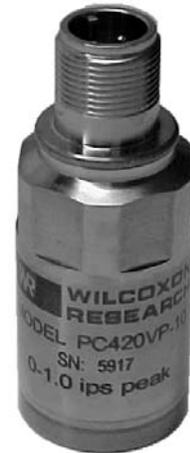
As the use of these loop-powered sensors has become popular the demand to be able to install and operate them in hazardous classified areas has also increased. 4-20 mA sensors are available as Intrinsically Safe certified units as well as in Explosion-Proof housings. This allows their use in those areas classified under NEC® section 500 as classified hazardous areas.
