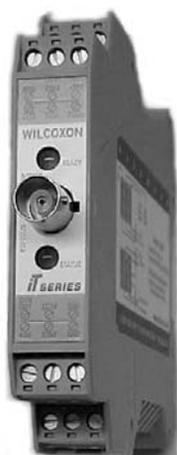
These modules offer more power and space for the signal processing than the sensor version. The transmitters can also implement stronger filtering with more filter options than the sensor. Whether the user wants to trend the entire vibration spectrum of signals or focus on a small range within the possible spectrum, the transmitter modules give more options for the user.
