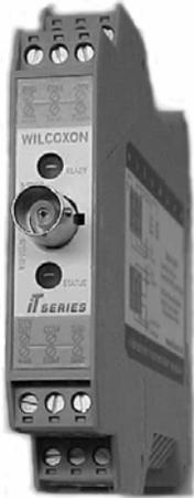
In some plants, accelerometers have already been installed permanently on machines to aid the vibration data collection process. These are often located on equipment in hard-to-reach areas or for safety reasons. These already existing sensors can also be used for gathering 4-20 mA vibration signals. The transmitters are powered from 24-Volt DC supplies and output a processed signal quite similar to that produced by the 4-20 mA sensors.
